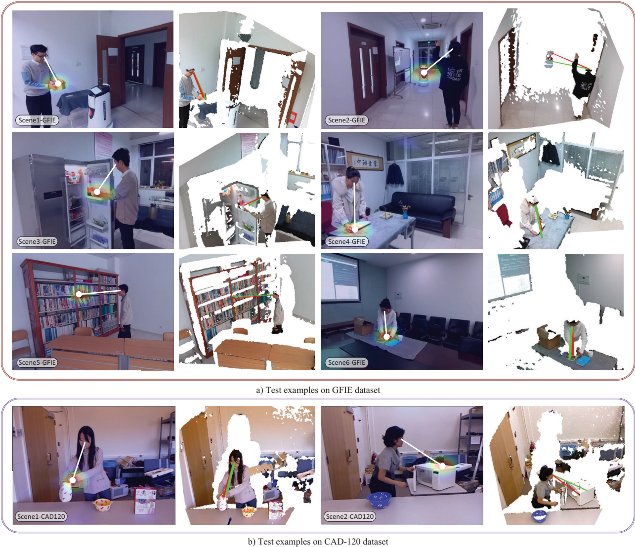
Figure 5. Visualization of test examples on GFIE and CAD-120 datasets. The endpoint of the white line indicates the gaze target in the image. The red and green lines in the point cloud represent the ground truth and sight line predicted by the GFIE model, respectively.
