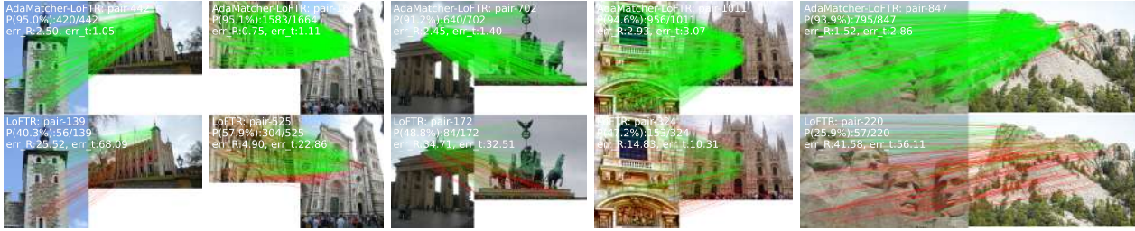
Figure 5. Qualitative results. AdaMatcher-LoFTR (top row) is compared to LoFTR (bottom row) in MegaDepth datasets. Matches with epipolar error beyond 1 \times 10^{-4} are shown in green lines, and the rest are shown in red. Under scale or viewpoint variations, AdaMatcher-LoFTR performs far superior to LoFTR.
