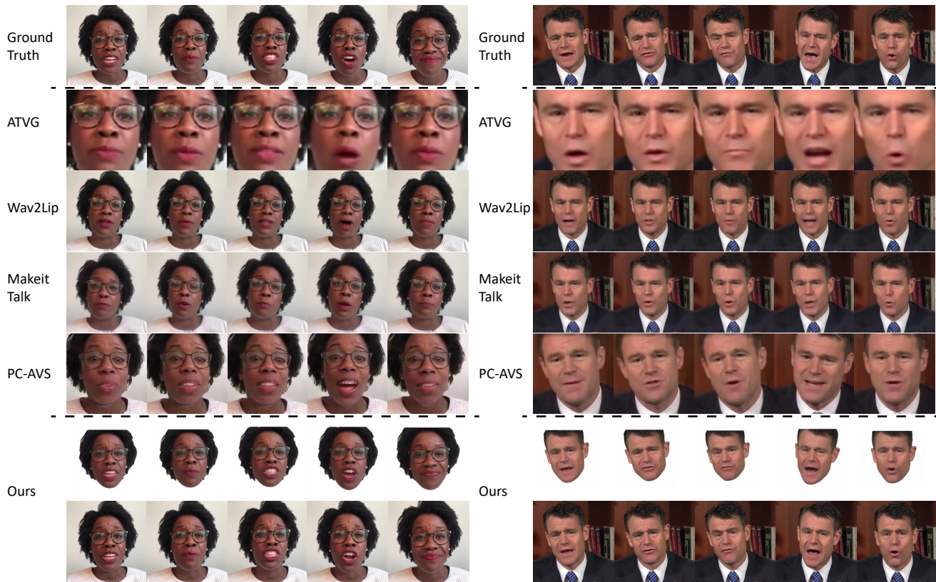
Figure 5. Qualitative comparison with ATVG [5], Wav2Lip [24], MakeitTalk [44] and PC-AVS [43]. Row 1 (Ground Truth): the corresponding video frames to the input audio. Last two rows (Ours): rendered face I_{face} and output image I (Fig. 2), respectively. The portraits generated by our method have highly synchronized lip movements and fine facial details (e.g., teeth and wrinkles) that preserve the target person’s identity well, thus outperforming all previous methods.
