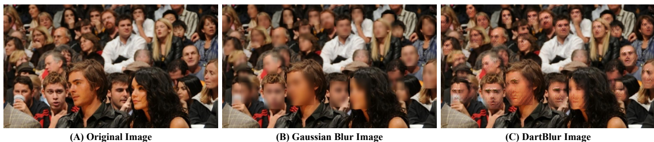
Figure 6. Example image anonymized with Gaussian blur and DartBlur. On top of Gaussian blur, DartBlur tends to adjust the contrast of the image and add special textures in key areas. Besides, DartBlur only uses Gaussian blur as the preprocessing tool so that accessibility can be guaranteed. Best viewed in color.
