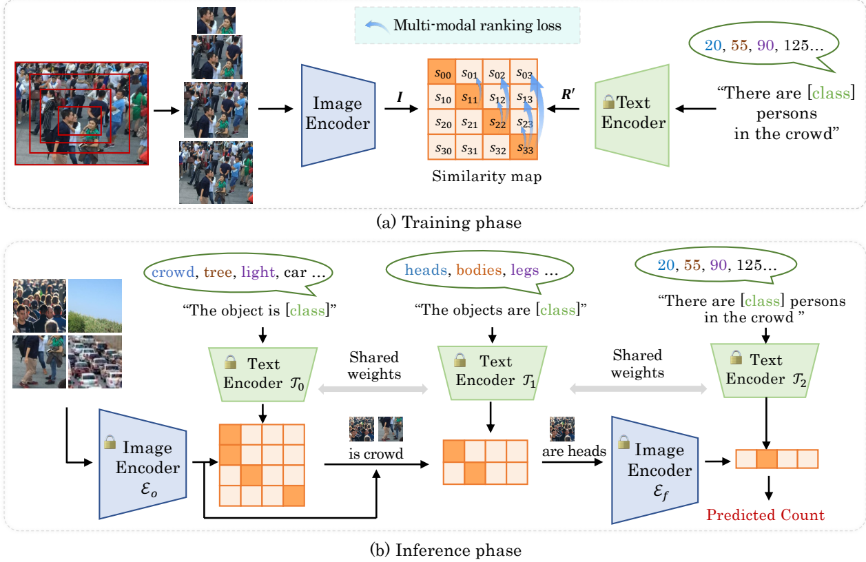
Figure 2. Overview of our framework. (a) During the training phase, we fine-tune the image encoder by introducing ranking prompts while the parameters of the text encoder are frozen. (b) During the testing phase, we propose a progressive filtering strategy that progressively queries the most likely crowd patches and maps the filtered patches into the specific quantitative count.
