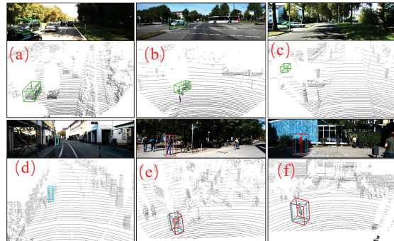
Figure 4. Qualitative analysis of pseudo labels on KITTI. For a better view, we only show the objects we are interested in and set the pseudo-labeling car, pseudo-labeling pedestrian, and ground truth bounding box in green, cyan, and red, respectively, whilst projecting boxes in point cloud back to RGB images. (a) and (b) show the case of category errors, (c) and (d) show the missing-annotated instance of the dataset, and (e) and (f) show the case of poorly localized pseudo labels. Best viewed in color.
