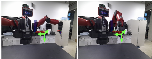
Figure 6. Snapshots of PBVS. The goal is to move the end-effector to the target pose (green). The figure on the right shows the robot configuration upon the convergence of PBVS.
