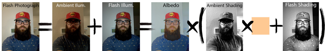
Figure 2. We can model the flash photograph formation in terms of separate shading maps for flash and ambient lights with a shared albedo.
