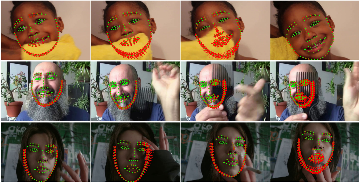
Figure 4. Example of ground truth labels (●) obtained semi-automatically from an ensemble of 45 models (▲). Ensembling these diverse models provides ground truth labels that do not flicker and can thus be used to measure flickering against. Note how landmark points with the most uncertainty are the most prone to having flickering predictions across consecutive frames.
