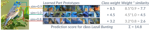
Figure 3. Example of local explanation of PIP-Net with only 3 prototypes for the correct class. PIP-Net learns part-prototypes visualized as patches from the training data, and localizes similar image patches in an unseen input image.
