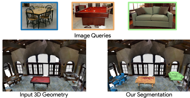
Figure 7. Image-based 3D Object Detection. A 3D scene (bottom left) can be queried with images from Internet (top) to find matching 3D points (bottom right). The colors of the image query outlines indicate the corresponding matches in the 3D point cloud. All 3 images are under Creative Commons licenses.
