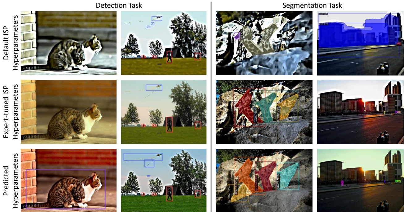
Figure 3. Image analytic vision tasks: Object Detection (left) and Image Segmentation (right) on COCO dataset. Default ISP hyperparameters (top), expert-tuned hyperparameters (middle), and the proposed method (bottom). The proposed method achieve better performance for downstream tasks.
