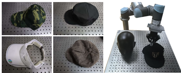
Figure 4. The real robotic testing platform includes a Ur5 robotic arm as the main body, an AG-95 parallel finger gripper, and a Realsense 435i depth camera. We evaluate the success rate with different random initialization.
