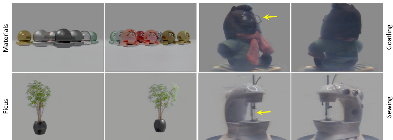
Figure 4. Reconstructions by our EventNeRF on synthetic (“Materials”, “Ficus”) and real (“Goatling”, “Sewing”) sequences. Our approach reconstructs specularities (“Materials”), thin structure (“Ficus”) and even the eyeglass frame and the needle from the “Goatling” and “Sewing” sequences respectively (see yellow arrow).
