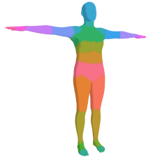
Figure 3. We split the SMPL model into 24 segments based on the blend weights. These segments help in determining the initial rotation estimate in the ARE pipeline. Here the segments are assumed to be rigid.
