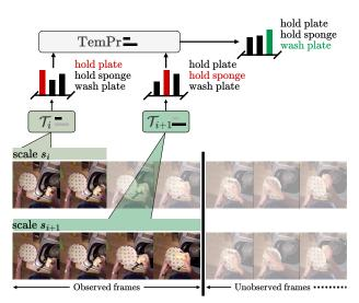
Figure 1. Early action prediction with TemPr involves the use of multiple scales for extracting features over partially observed videos. Encoded spatio-temporal features are attended by distinct transformer towers ( $\mathcal{T}$ ) at each scale. We visualize two scales, where the fine scale  $\mathcal{T}_i$  predicts 'hold plate', and the coarse scale  $\mathcal{T}_{i+1}$  predicts 'hold sponge'. Informative cues from both scales are combined for early prediction of the action 'wash plate'.
