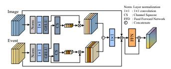
Figure 3. The Event-Guided Adaptive Channel Attention module. The channel weights for the image branch are extracted from the event branch.
