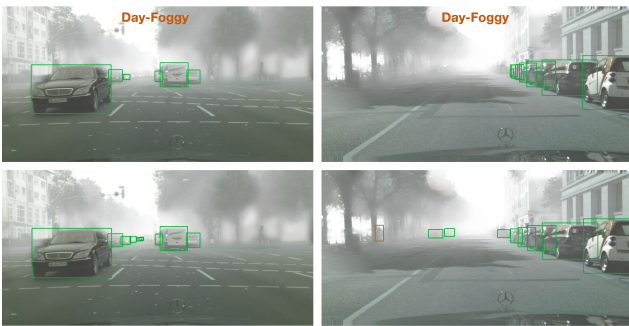
Figure 5. Qualitative Results. In the foggy scenes, the objects further away w.r.t the camera are more obscure than the near ones. Due to this FasterRCNN (Top) struggles to detect them. car and person missed by FasterRCNN are successfully recovered by our approach (Bottom).
