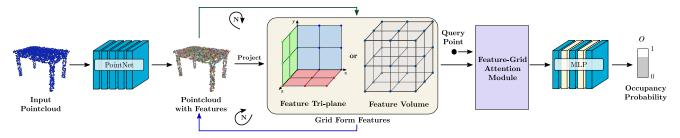
Figure 2. An overview of our method. Given input surface points, we obtain an implicit occupancy field with iterative alternation between features in the forms of points and 2D or 3D grids (Sec. 3.2). Then we decode the occupancy values for query points with a learned attention-based interpolation from neighboring grids (Sec. 3.3).
