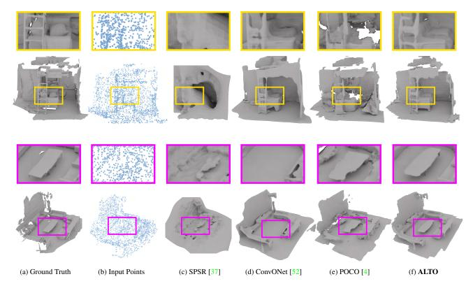
Figure 8. Cross-dataset evaluation of ALTO and baselines by training on Synthetic Rooms [52] and testing on real-world ScanNet-v2 [14]. Note the large conference-room table is missing in ConvONet [52] (purple inset). The ladder (yellow inset) is a high-frequency surface and we believe our method is qualitatively closest. Please zoom in if browsing with PDF.
