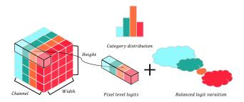
Figure 2. Diagram of the introduction of balanced logit variation, where we perturb the per-pixel logit with a category-specific noise. The noise variance is in inverse proportion to the category scale.
