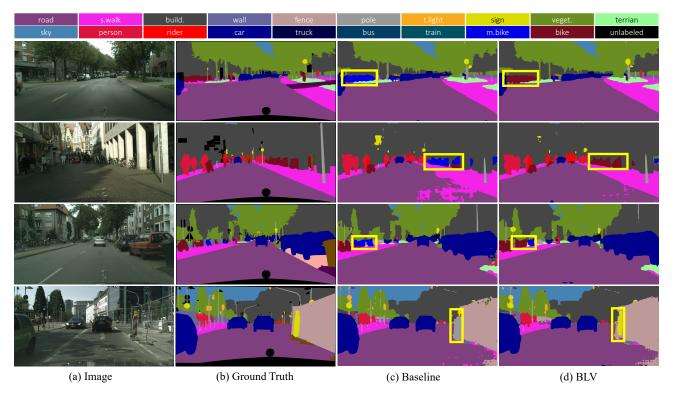
Figure 4. **Qualitative results on Cityscapes val set**. Baseline and BLV are trained on  $GTA5 \rightarrow Cityscapes$  benchmark of unsupervised domain adaptive semantic segmentation task. (a) Input images. (b) Ground truth annotations for the corresponding images. (c) Result of the DAFormer baseline. (d) Result of our method (DAFormer + BLV). Yellow rectangles highlight the promotion of segmentation results by our method on tail categories.
