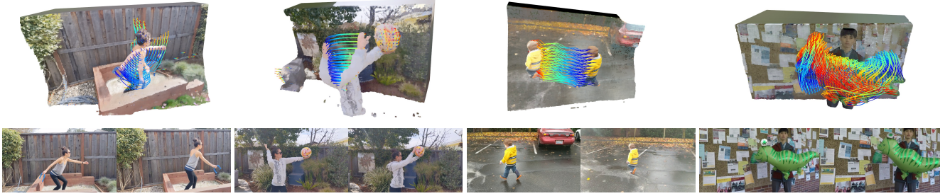
Figure 5. 3D visualizing of trajectories computed by integrating velocity fields v(\mathbf{p}; t) from equation (5). Trajectories are colored to represent temporal order, and overlaid with colored point clouds extracted from the optimized deformable NeRF. Bottom row shows two frames from each of the input videos.
