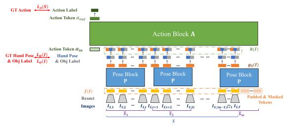
Figure 2. Overview of our framework. Given input video S, we first feed each image to a ResNet feature extractor, and then leverage short-term temporal cue via **P** applied to shifted windowed frames, to estimate per-frame 3D hand pose and object label. We finally aggregate the long-term temporal cue with **A**, to predict the performed action label for S from the hand motion and manipulated object label. We supervise the learning with GT labels.
