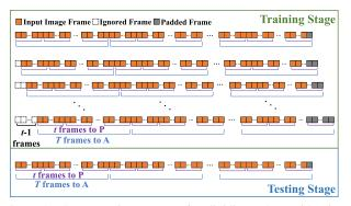
Figure 3. Segmentation strategy for dividing a long video into inputs of **HTT**. In the testing stage, we start from the first frame, while in the training stage, we offset the starting frame within t frames to augment the training data diversity.
