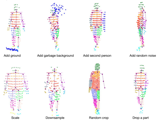
Figure 4. Data augmentations applied to the synthetic point clouds (colored by ground truth segmentation labels). Ground truth skeletons are shown in purple. Background points are in blue.
