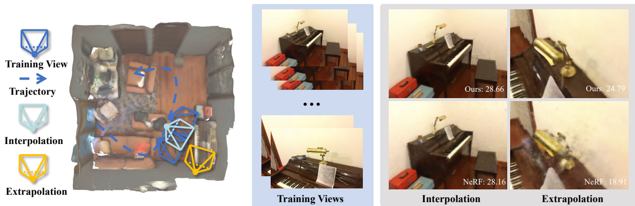
Figure 1. Illustration of the free view synthesis task. Free view synthesis aims at synthesizing photo-realistic images on both interpolation and extrapolation setting. In this paper, we propose a novel method, NeRFVS, based on the neural radiance field (NeRF) [12] to achieve indoor scene free view synthesis. Our NeRFVS significantly reduces the distortions and floaters (as also evidenced by the PSNR numbers), producing high-quality images on interpolation and extrapolation setting.
