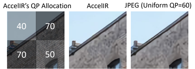
Figure 9. Block artifact comparison between AccelIR and JPEG of blocks greatly varies according to QP, which critically affects the amount of edgy components across the image blocks. In contrast, in non-IR tasks, the favorable region is fixed, which is determined by target objects (e.g., cars).
