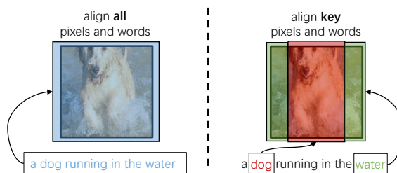
Figure 4. Left: Aligning all pixels and words. Right: aligning key entity words (dog and water) with local regions (in red and green).
