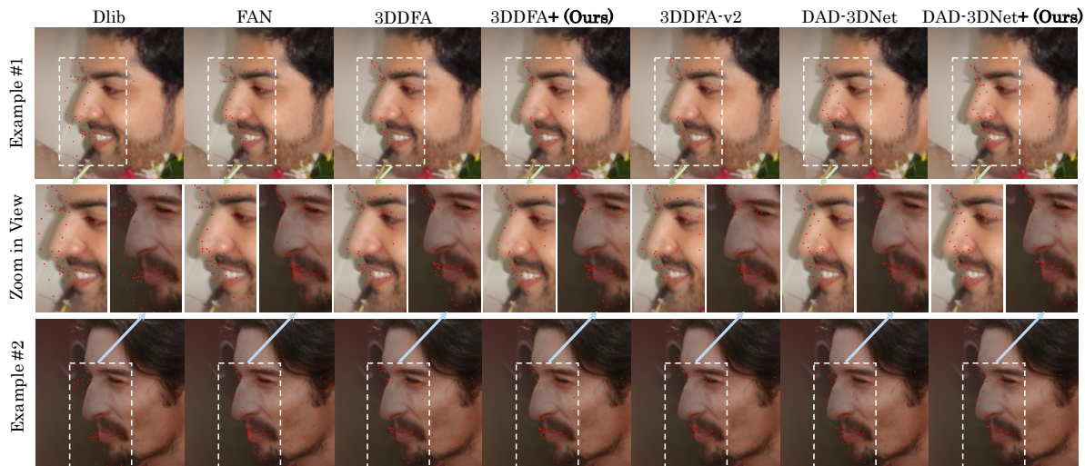
Figure 5. The visual results of Dlib [31], FAN [5], 3DDFA [22], our refined 3DDFA+, 3DDFA-V2, DAD-3DNet [34], and our refined DAD-3DNet+ on images randomly sampled from DAD-3DHeads [34] testing set. We show the enlarged error region (while box) in the middle row.
