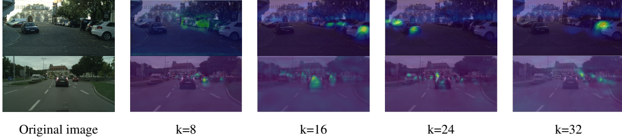
Figure 4. Visualization of generated weight in SMF for each group. We take two sample images from validation set of Cityscapes, which are shown in the first column. For each image, we sample 4 groups from the total 32 groups and highlight the generated attention over each sample image as shown in columns 2 to 5, respectively. We can observe that the generated weight in different groups detect different foreground regions effectively. k denotes the k^{th} group defined in Section 4.
