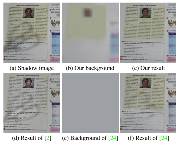
Figure 1. Document image shadow removal. With the assumption of constant background, results of [2] and [24] may cause color distortion or shadow remnant. By using a spatially varying background, our method can produce more desirable result.
