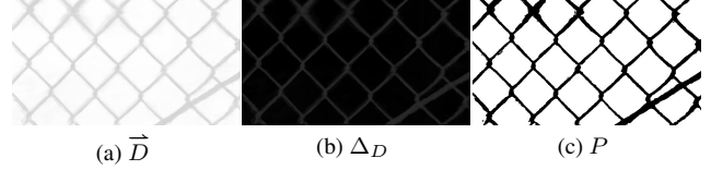
Figure 2. An illustration of the depth and mask used for selective supervision (without losing generality, we show the example for fence, and this applies to other types of occlusions as well): (a) estimated depth ( \vec{D} ) of the scene with occlusion, (b) the bidirectional depth difference ( \Delta_D ), and (c) the supervision mask ( P ). Note that the white regions in (c) denote the desired background details that need supervision and undesired foreground occlusions are marked in black. Please visit our project page for animated results.
