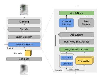
Figure 4. The architecture of RoDLA model. RoDLA is comprised of Encoder, Query Selection, Decoder, and Matching components. It optimizes the attention mechanism in Encoder, heightening focus on crucial tokens and reinforcing key token connections in multi-scale features to extract stable features.
