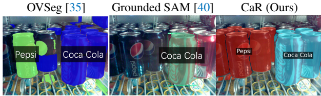
Figure 2. Our method CaR can fully inherit the vast vocabulary space of CLIP , by directly using features from a pre-trained VLM, i.e. , CLIP, without any fine-tuning. Although the scene in the image is simple, state-of-the-art methods fine-tuned on segmentation datasets [35, 40] fail to segment and recognize Pepsi and Coca Cola correctly.
