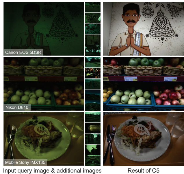
Figure 1: Our C5 model exploits the colors of unlabeled additional images captured by the new camera model to generate a specific color constancy model for the input image. These additional images can be randomly loaded from the photographer’s “camera roll”, or they could be a fixed set taken once by the camera manufacturer. The shown images were captured by unseen DSLR and smartphone camera models [38] that were not included in the training stage.
