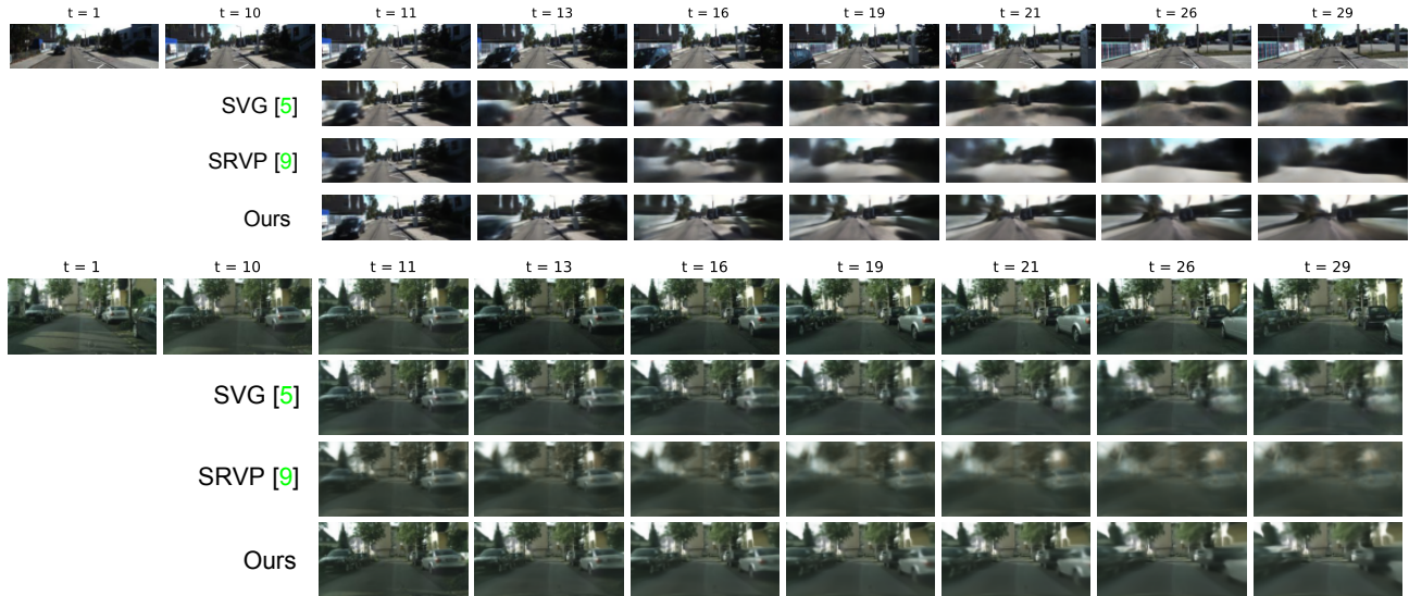
Figure 9: Qualitative Comparison. We compare SLAMP to SVG [4] and SRVP [8] on KITTI ( top ) and Cityscapes ( bottom ). Our model can better capture the changes due to ego-motion thanks to explicit modeling of motion history.
