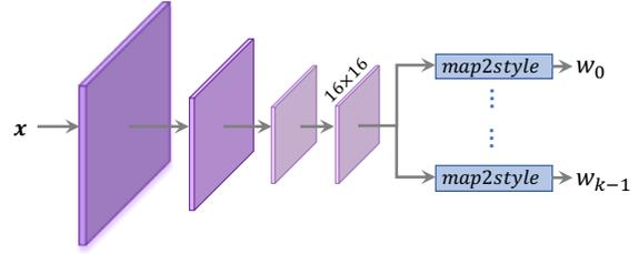
Figure 3. Our simplified encoder architecture. All  $k$  input style vectors of the generator are extracted from the encoder’s final  $16 \times 16$  feature map which is passed through  $k$  *map2style* blocks [35].
