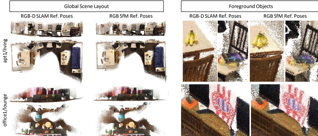
Figure 6. Consistency of depth map fusion for 12Scenes [74]. Left: RGB-D SLAM pseudo GT leads to a significant warp of the global scene layout, which is clearly reduced by the SfM pseudo GT. Right: Foreground objects appear blurred for SfM pseudo GT poses compared to the sharper depth alignment generated by RGB-D SLAM pGT.
