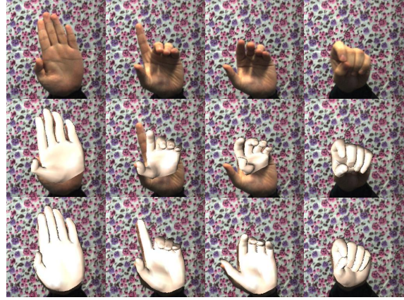
Figure 4. Comparison of the experimental results on the STB dataset [16] before and after self-supervised training with our model. The first row is the input RGB image. The second row is the results of directly test on STB dataset with pre-trained model on FreiHAND dataset. The third row is the results after our self-supervised training with the proposed model (binocular version).
