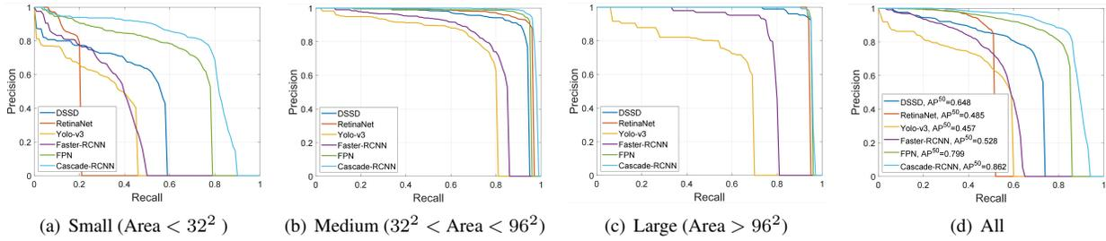
Figure 9. PR (precision-recall) curves of different object detection algorithms on the test set of FloW-Img (IoU threshold = 0.5).  $AP^{50}$  denotes the average precision with the IoU threshold at 0.50.
