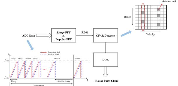
Figure 5. Conventional FMCW radar signal processing chain.
