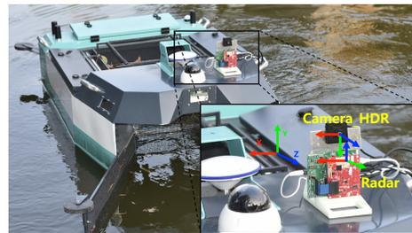
Figure 4. Our acquisition platform is equipped with two cameras and a millimeter wave radar. The directions of the sensors used in collecting the FloW-RI are marked in different color (X-red, Y-green, Z-blue).
