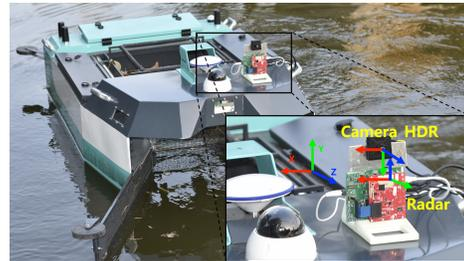
Figure 4. Our acquisition platform is equipped with two cameras and a millimeter wave radar. The directions of the sensors used in collecting the FloW-RI are marked in different color (X-red, Y-green, Z-blue).
