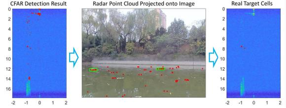
Figure 7. The annotation processes. In the first image, the red points on the RDM image show the cells detected by the CFAR detector with a low threshold. The second image shows the corresponding points projected on the RGB image, and the real target points are annotated (framed by the green boxes). Last image shows the final real target cells in red.
