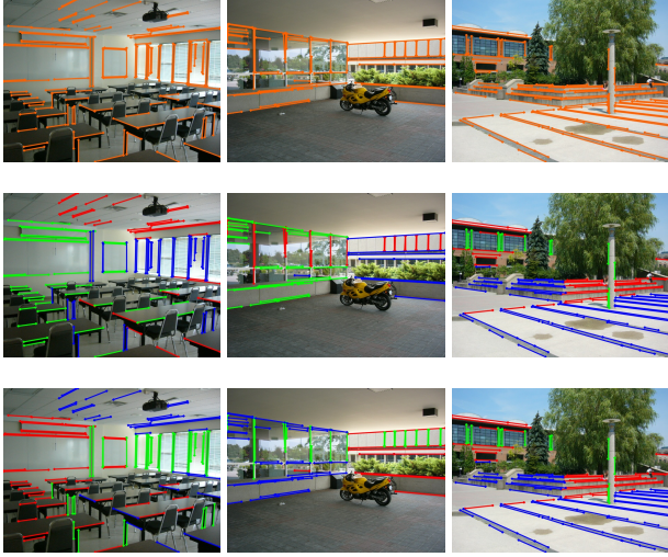
Figure 5. Some example images obtained by the exhaustive BnB and the proposed method on YUD [18]. The first row shows the example images with extracted lines. The second row shows the line classification results of the exhaustive BnB. The third row shows the line classification results of the proposed method.
