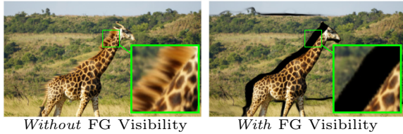
Figure 3: Foreground Pixel Visibility. Rendering an RGBD layer without pixel visibility (left) leads to stretchy triangles, whereas rendering with pixel visibilities (right) enables seeing through to the background (represented with black pixels here).
