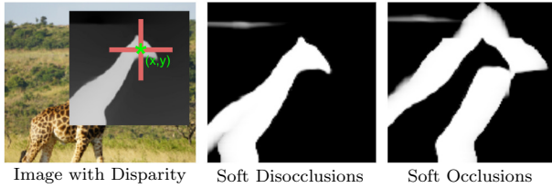
Figure 4: Soft Disocclusions and Occlusions. At each point (x, y) in an image, we compare disparity differences across horizontal and vertical scan lines to compute soft disocclusion and occlusion maps.
