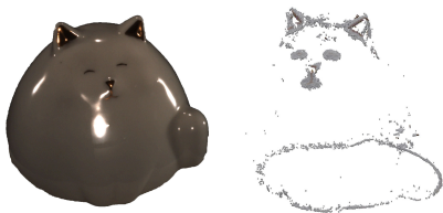
Figure 9: Reconstruction result using COLMAP [24, 25] on photographs with 4 point lights, for more shading cues compared with a full-on pattern. The left image is a photograph, and the right geometric reconstruction. The accuracy is 34.8% and the completeness is 5.6%.
