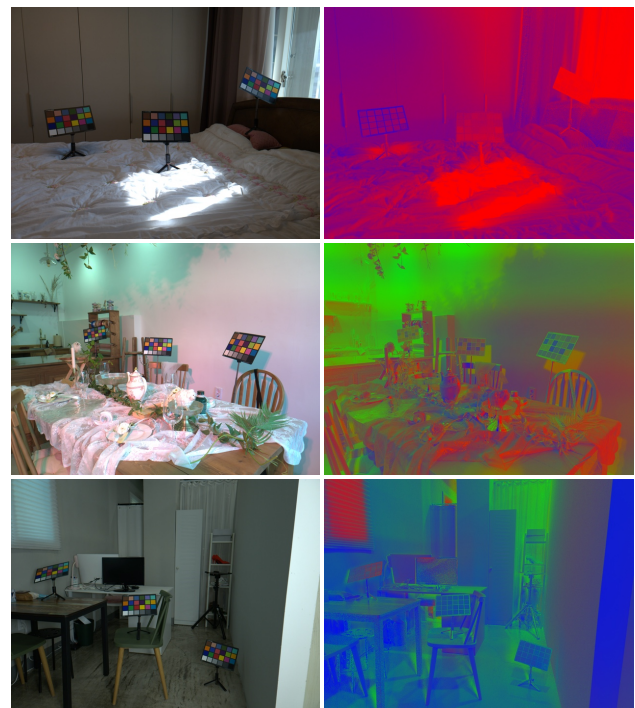
Figure 1. Two and three-illuminate scene samples from LSMI dataset (left) and illuminant coefficient maps that show the ratio of how illuminants are mixed per pixel (right). Raw images are converted to the sRGB space with an auto white balance for visualization purposes.
