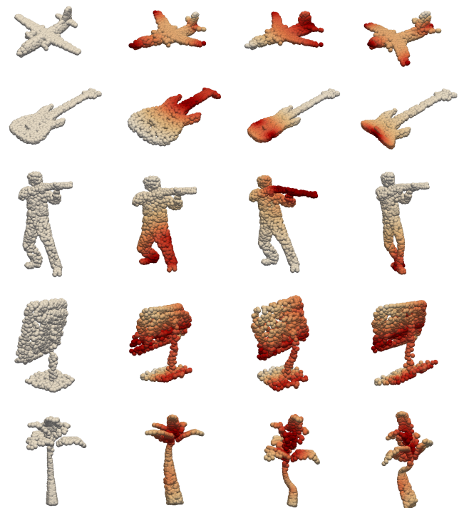
Figure 1. Locally augmented point clouds using PointWOLF. In each row, the left most sample is the original, and the remaining samples are its locally transformed results (brighter regions indicate stronger local transformations). PointWOLF can locally transform objects while preserving the original shape identity.
