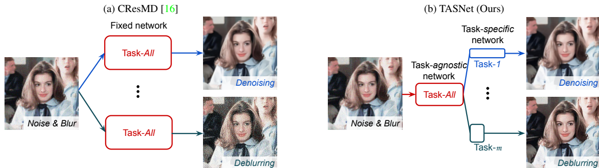
Figure 2: The overview of our efficient architecture for controllable image restoration. (a) CResMD [16] has a fixed network across all tasks and requires separate inference through the full model whenever the target restoration task becomes different. (b) Our task-agnostic and task-specific network (TASNet) shares the early layers to facilitate feature reuse. When we perform inference for multiple tasks, the task-agnostic part requires only a single computation, of which the output feature can be reused multiple times as the input for the task-specific network. The architecture of the task-specific network is adaptively adjusted for each given task. The width and the height of boxes represent the number of layers and channels of neural networks, respectively. In this example, two popular restoration tasks of denoising and deblurring are visualized, where different colors represent the corresponding inference path.
