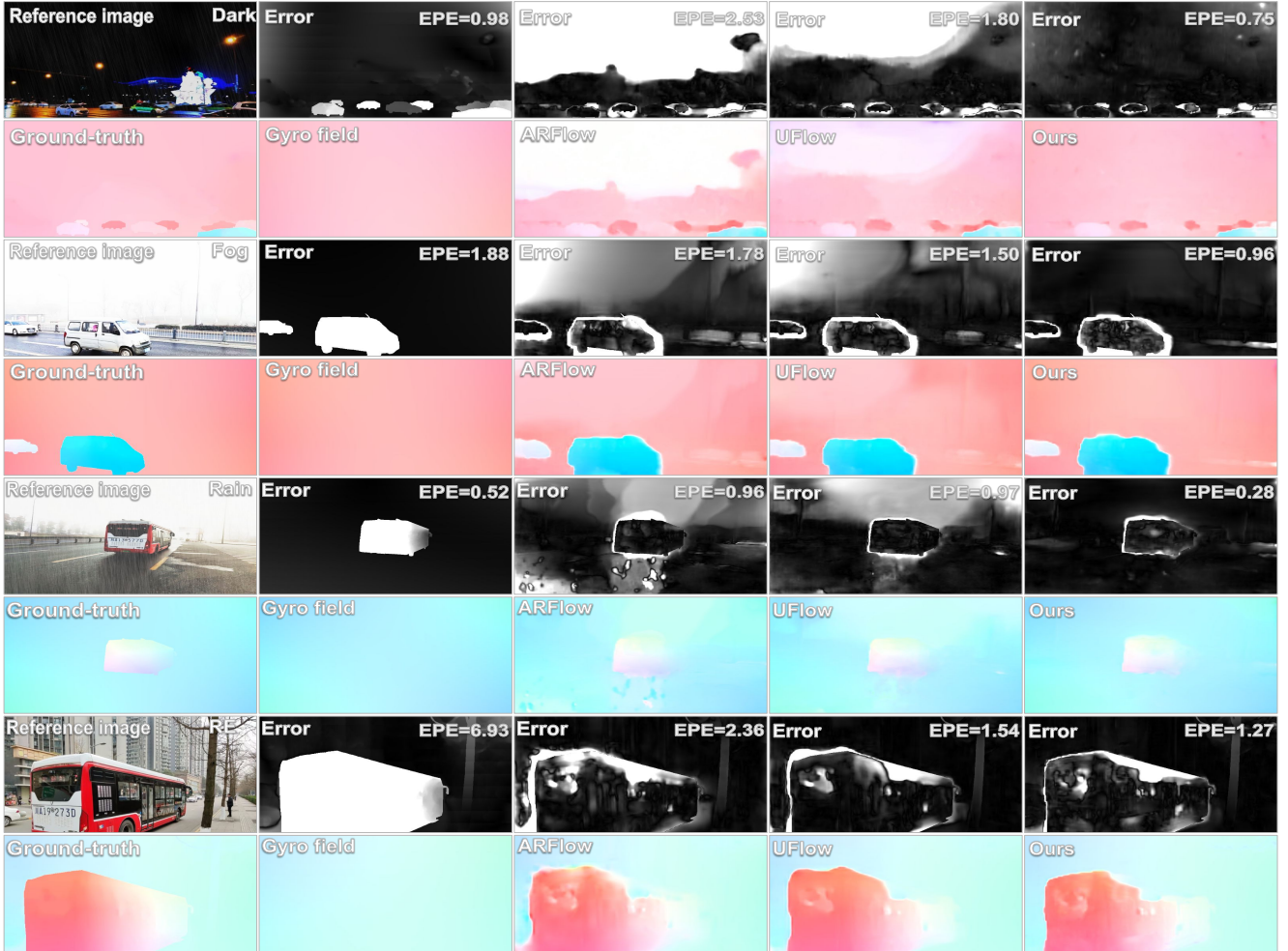
Figure 7. Visual comparison of our method with gyro field, ARFlow [30], and UFlow [19] on the GOF evaluation set. For the first 3 challenging cases, we notice that our method achieves convincing results by fusing the background motion from the gyro field and the motion details from the optical flow. For the last example, in regular scenarios, fusing gyro field helps the learning of optical flow where the network produces accurate and sharp flow around the boundary of objects.
