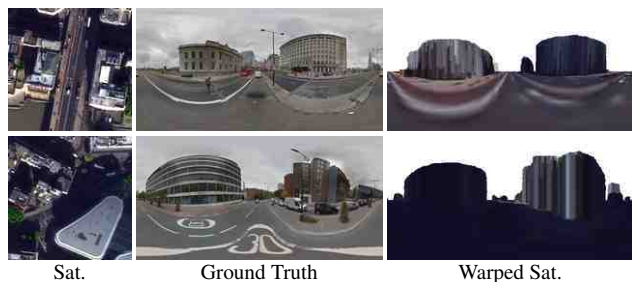
Figure 6: Warped color satellite information. The examples illustrate the low-quality of warped satellite images which often do not provide useful color information.
