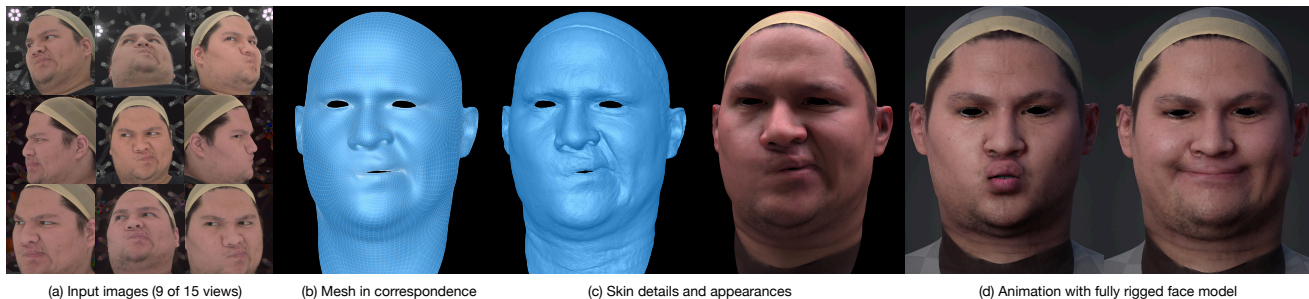
Figure 1: Given (a) multi-view images, our face modeling framework ToFu uses volumetric sampling to predict (b) accurate base meshes in consistent topology as well as (c) high-resolution details and appearances. Our efficient pipeline enables (d) rapid creation of production-quality avatars for animation.
