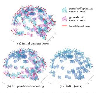
Figure 5: Visual comparison of the initial and optimized camera poses (Procrustes aligned) for the *chair* scene. BARF successfully realigns all the camera frames while NeRF naïve positional encoding gets stuck at suboptimal solutions.
