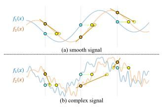
Figure 2: **Predicting alignment from signal differences.** Consider two 1D signals where  $f_1(x) = f_2(x + c)$  differs by an offset c. When solving for alignment, smoother signals can predict more coherent displacements than complex signals, which easily results in suboptimal alignment.
