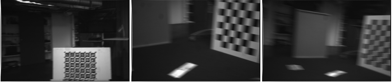
Figure 5. Examples images from the proposed dataset for benchmarking visual odometry from motion blurred image sequences. The dataset contains multiple sequences with varying levels of motion blur.
