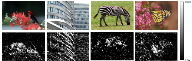
Figure 7: Variance of learned dynamic high-pass kernel from the 4 th residual block, 5 th group. The kernel correctly learns to filter high-frequency details such as sharp pixel value transitions.
